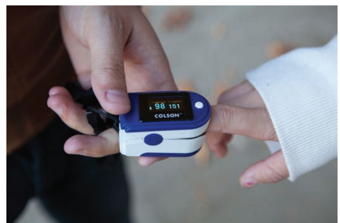
Figure 29–26 ■ Fingertip oximeter sensor (cordless). Amelie-Benoist/BSIP/Alamy.
