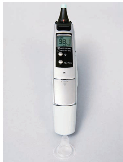
Figure 29-8 ■ An infrared (tympanic) thermometer used to measure the tympanic membrane temperature.
